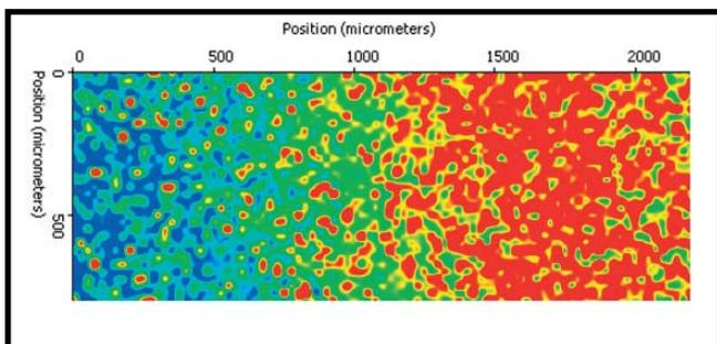
**Figure 3: A 750 x 2,250 micron, two-dimensional map of a sample of silicon deposited on glass. The chemical image was generated by calculating the ratios of the peak heights at 521 and 480 cm-1 at each point on the map. Crystalline areas are shown in red and amorphous in blue.**
