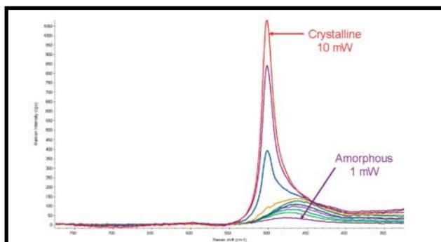
**Figure 4: The effect of excitation laser power on amorphous silicon. The 532 nm excitation laser power at the sample was controlled by the DXR Raman microscope laser power regulator and was increased in 1 mW steps from 1 to 10 mW. Results show little effect on the amorphous silicon at power levels up to 4 mW. Higher laser power progressively converts the amorphous silicon to the crystalline form.**
