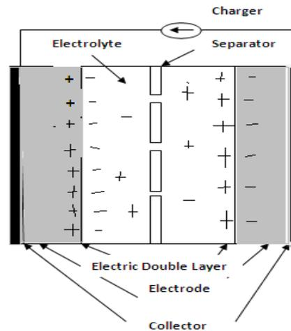
Fig 6 Ultracapacitors [10]
