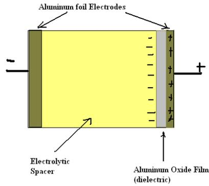
Fig 5 electrolytic capacitors [9]
