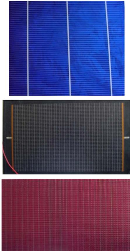
Figure 2. Crystal-Si and thin-film *flexible* solar cells
