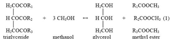
In this reaction, a catalyst is needed in order to improve the reaction rate. Conventionally, alkaline metal alkoxides are the most effective methanolysis catalyst compared to the acidic catalyst. Sodium alkoxides are the most efficient catalyst used for it, although KOH and NaOH can also be used (Meher, et.al., 2006). Methanolysis occurs faster in the presence of a alkaline catalyst than that catalysed by the same amount of acid catalyst.
