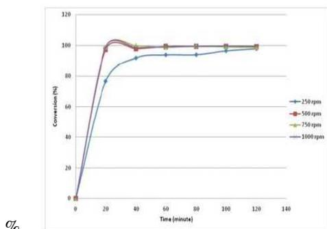
Fig. 4. Effect of stirring speed (rpm) on % conversion of oil (50 °C, M=4.5, C= 4 %)
