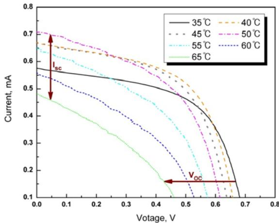
Fig. 7 Comparison of I-V curve due to temperature change
