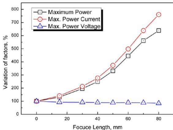
Fig. 10 Performance changes due to focus length
