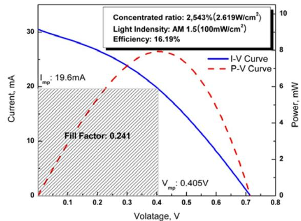
Fig. 9 I-V curves of DSSC due to Focus length
