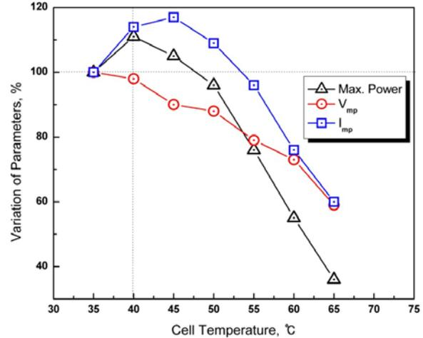
Fig. 8 Performance changes due to temperature change
