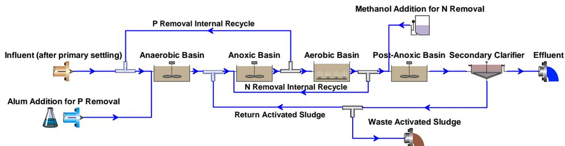
**Fig. 1** Process Flow Diagram of A Traditional Biological Nutrient Removal Process. Two internal recycle streams and one RAS stream for nitrogen and phosphorus removal.)
