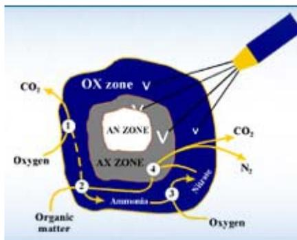
**Fig. 3** NADH Probe in the SymBio<sup>®</sup> Process for Simultaneous Nitrification and Denitrification When the dissolved oxygen is below 1.0mg/l in the bulk mixed liquor, oxygen gradients are created in the biological flocs, forming anaerobic zone (AN), anoxic zone (AX), and aerobic zone (OX) inside to accomplish simultaneous nitrification and denitrification.
