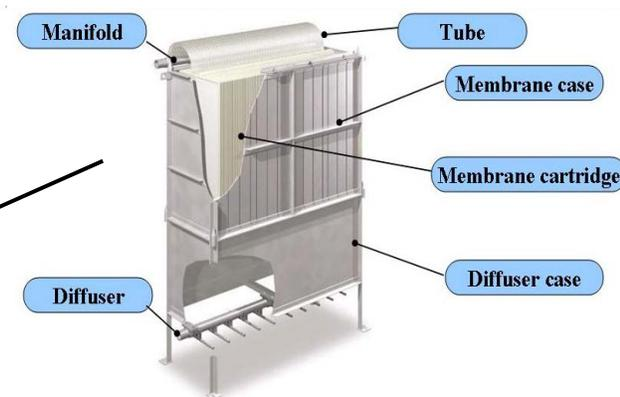
**Fig. 4** MBR Basin with Installed Submerged Membrane Units (Left), and Schematic Diagram of A Submerged Membrane Unit (Right).
