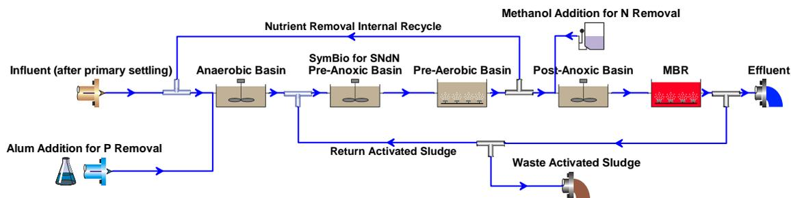
**Fig. 2** Process Flow Diagram for Enviroquip MBR for Enhanced Nutrient Removal. The SymBio process requires only one internal recycle stream is required for nitrogen and phosphorus removal.
