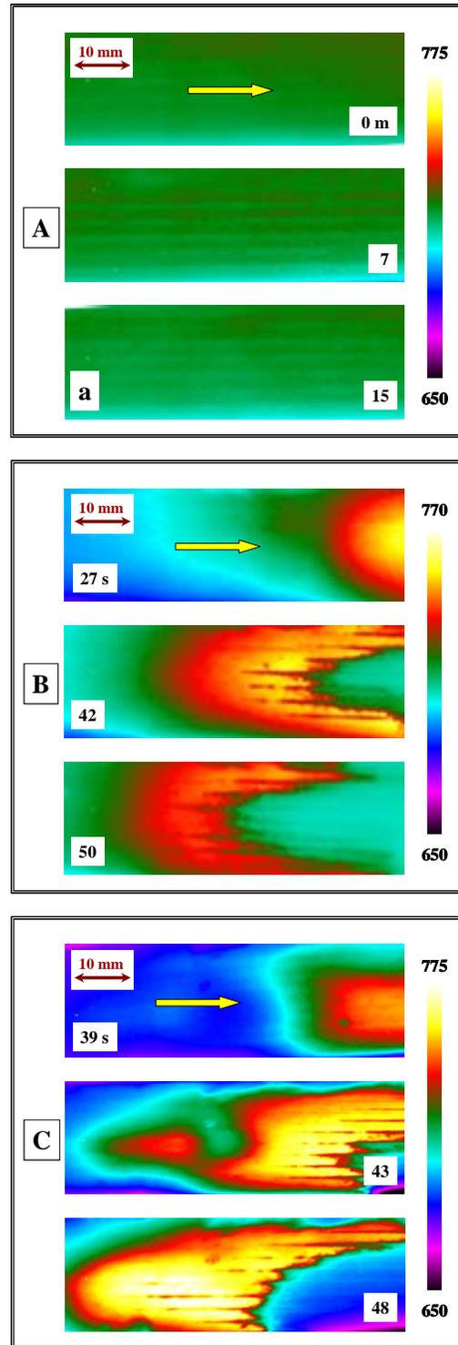
Figure 2: Thermal images of soot regeneration for soot loading of 10 g/L. Feed oxygen concentration (a) 5 v. %; (b) 12.5 v. %; (c) 15 v. %.
