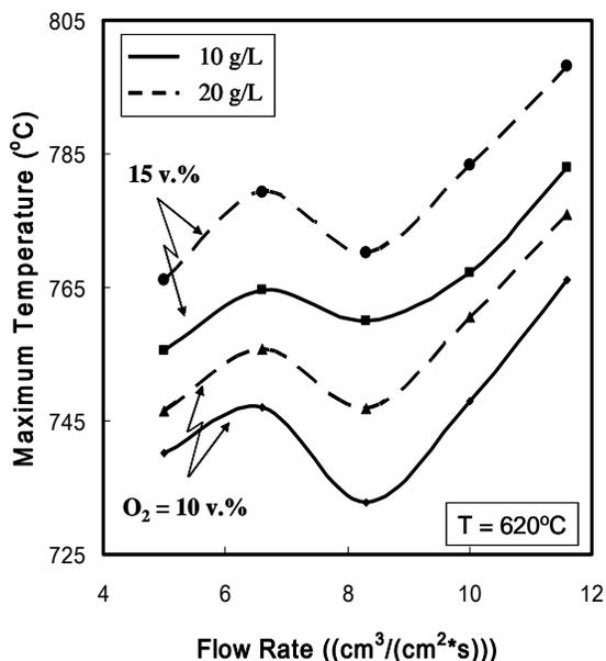
Figure 5: Impact of filter wall flow rate on maximum front temperature at several O<sub>2</sub> concentrations and soot loading of 10 and 20 g/L, feed temperature of 620 °C.
