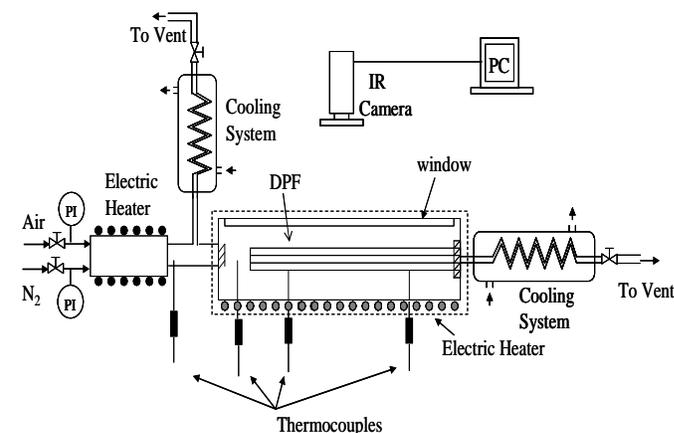
Fig.1. A schematic of the experimental system
