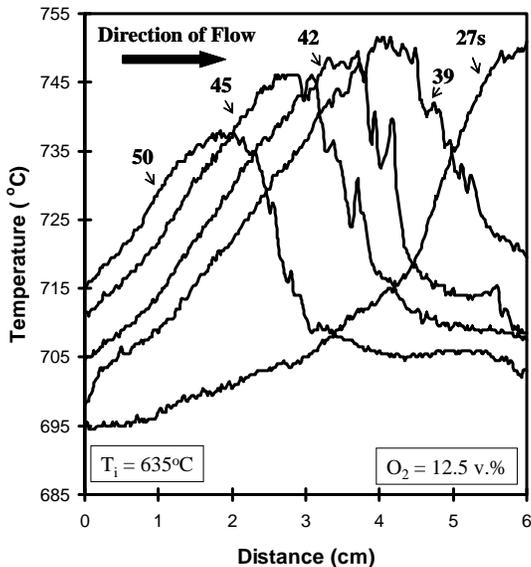
Figure 3: Moving temperature profiles originating from end of DPF. Soot loading of 10 g/L and  $O_2=12.5$  v. % (same experiment as that in Fig. 2, a).
