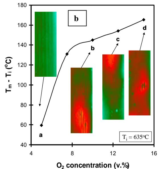
Figure 4: (a) Effect of oxygen concentration on the relation between maximum front temperature and its propagation velocity. Soot loading of 10 g/L; (b) Dependence of the maximum temperature rise on the oxygen concentration for soot loading of 20 g/L.
