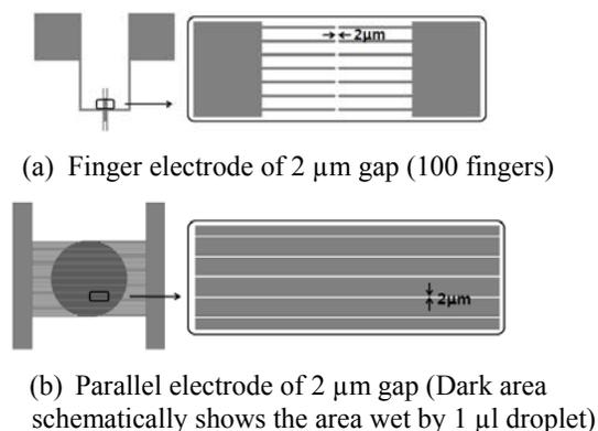
Figure 2: Schematics of electrode devices
