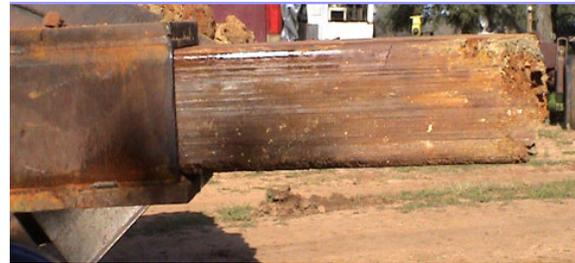
Figure 2: Continuous extrusion of compressed earth from small proof-of-concept machine.
