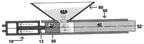
Figure 1: Schematic of compressed earth block extruder [11].
