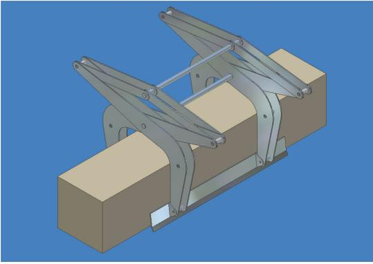
Figure 3: Isometric view of CEB lifter.
