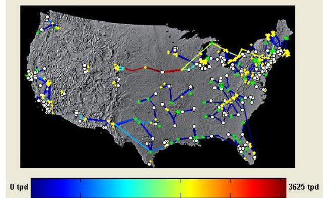
**Figure 1: Location of Economically Utilized Resources and H<sub>2</sub> Pipeline Network**
