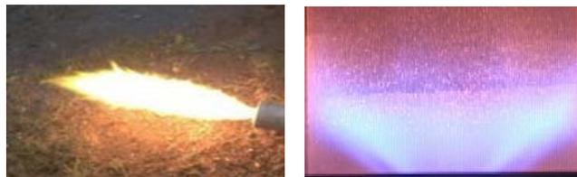
Figure 1: Conventional liquid fuel spray diffusion flame (left) and typical lean, premixed natural gas flame (right).
