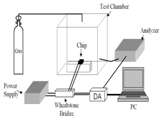
Figure 3 Shows the schematic of Experimental Test Bed. The test bed consists of glass test chamber in which the nanocomposite is tested, an chemiluminescence NO<sub>x</sub> analyzer which is used for monitoring the NO<sub>2</sub> concentration level in the test chamber and electrical circuit which is used for monitoring the change in electrical resistance of the nanocomposite when it is exposed to NO<sub>2</sub>.
