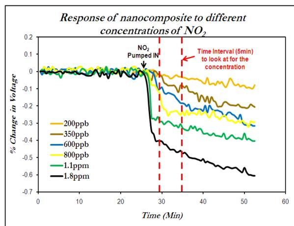
Figure 4 The response of nanocomposite to various concentrations of NO<sub>2</sub>. It is observed that the resistance of the nanocomposite decreases with increase in the NO<sub>2</sub> concentration.
