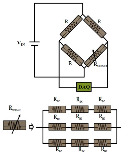
Figure 2. The equivalent circuit of the entire experimental setup and equivalent resistance of the nanocomposite. The resistor  $R_{\text{sensor}}$  in the Wheatstone bridge circuit is the resultant resistance of the nanocomposite.
