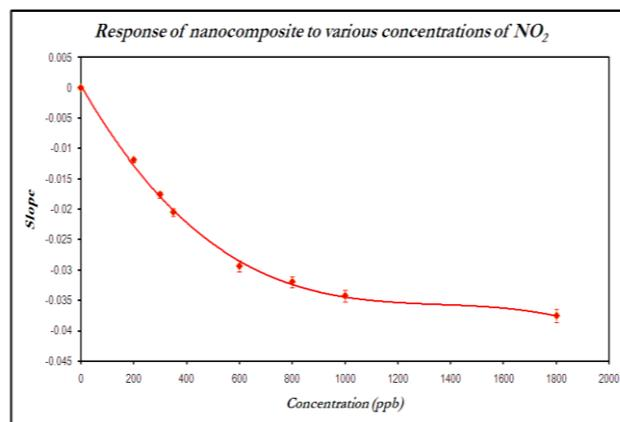
Figure 5 Slope vs. Concentration curve of the nanocomposite response to NO<sub>2</sub>. From the curve it is inferred that there is a quadratic response of the nanocomposite to NO<sub>2</sub>.
