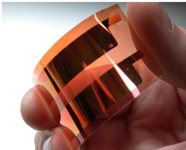
Fig. 1: Prototype of a flexible organic solar cell
