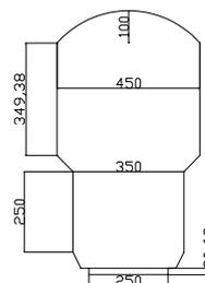
Figure 1: Piezo-electric transducer used for ultrasonic sonication treatment (scale 10 units = 1mm).
