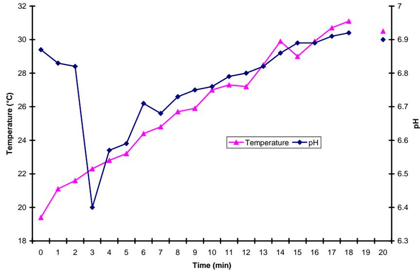
Figure 2: Temperature and pH variation during 1 MHz ultrasound sonication.
