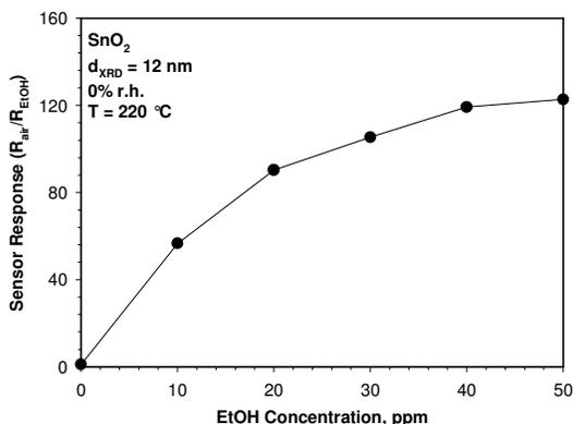
**Figure 2:** Sensor response to increasing ethanol concentrations.
