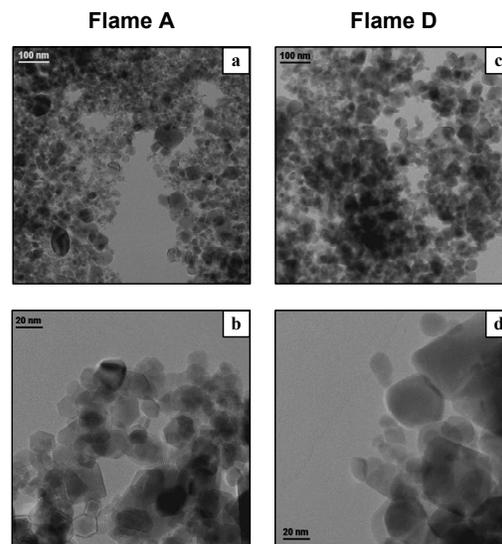
**Figure 1:** TEM images of SnO<sub>2</sub> particles produced by FSP. The particle size increases with increasing flame enthalpy.
