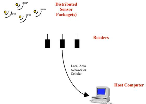
Figure 2. 3-tier architecture for an RF-enabled system
