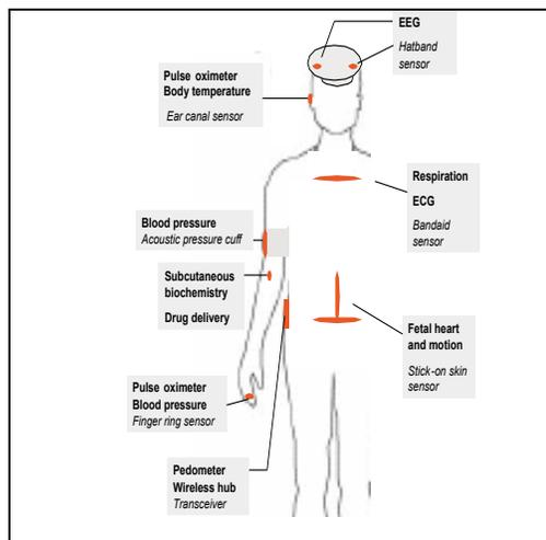
Figure 1. *Wearable Body Network with Biosensors and Transceiver.*
