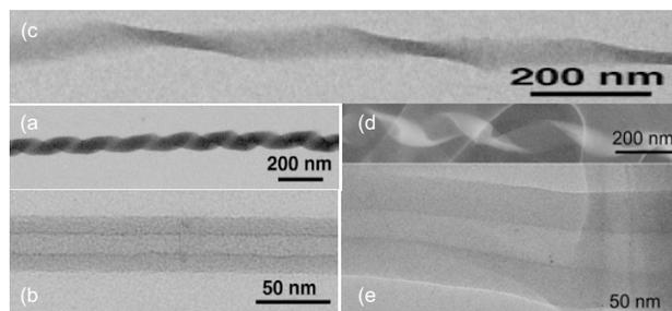
**Figure 1.** TEM images of (a) an individual helically coiled nanofiber from cardanyl glucoside mixtures, **1** (b) an individual nanotube from cardanyl glucoside mixtures, **1**. (c) a helically twisted nanofiber from saturated glucoside, **2**, and TEM images of self-assembled morphologies of DAP lipids, **3** in water, (d) helical coiled fibers and (e) nanotubes. The dimensions of the nanotubes were uniform and reproducible.
